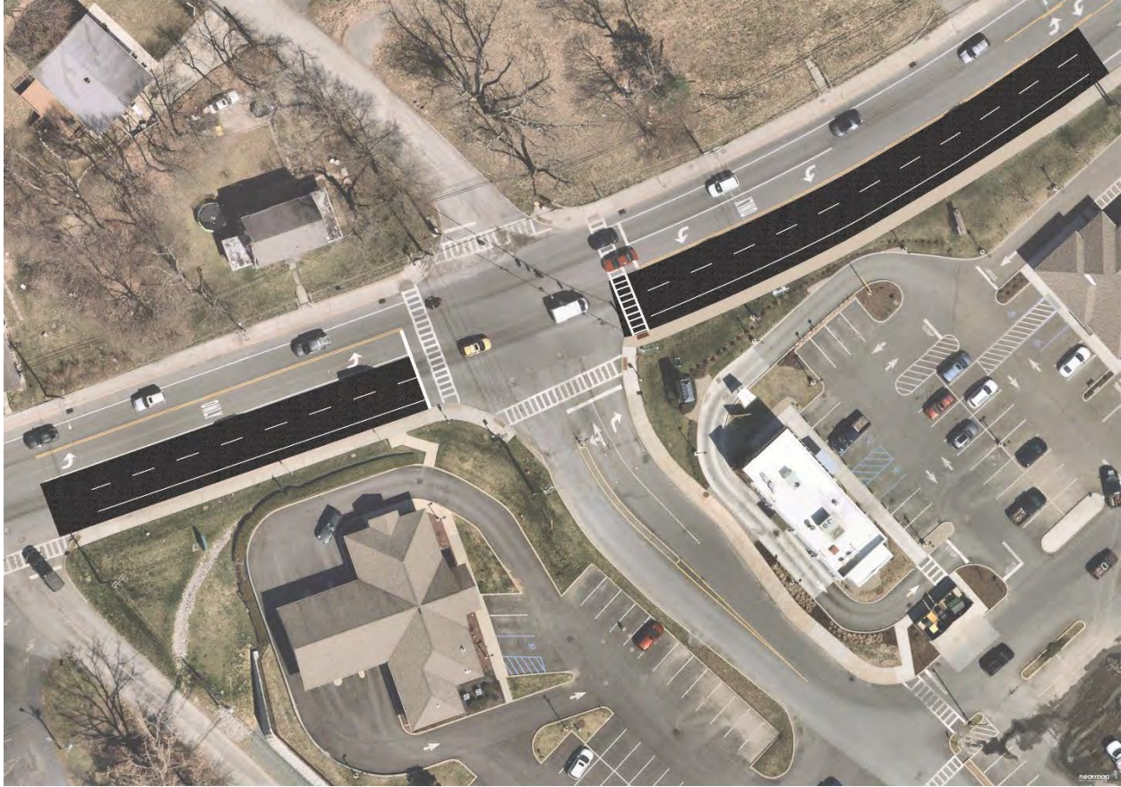
FIGURE 3.4: HOOSICK ROAD WIDENING AT ROOSEVELT AVENUE
