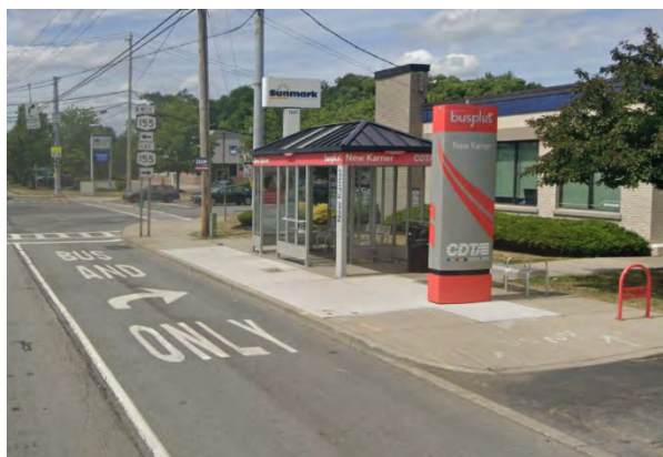
FIGURE 3.8: BUS TURNOUT EXAMPLE
